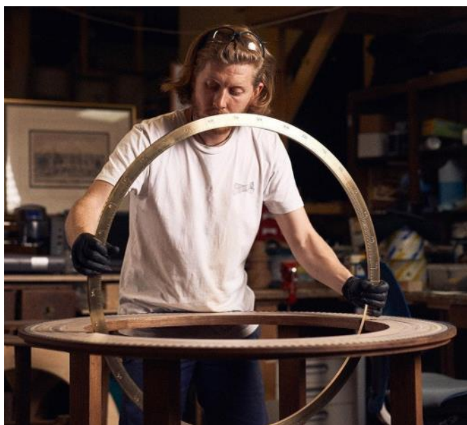
Figure 2. Fitting a Meridian. Image courtesy of Bellerby Globe-makers, Toby Essex, photographer.
