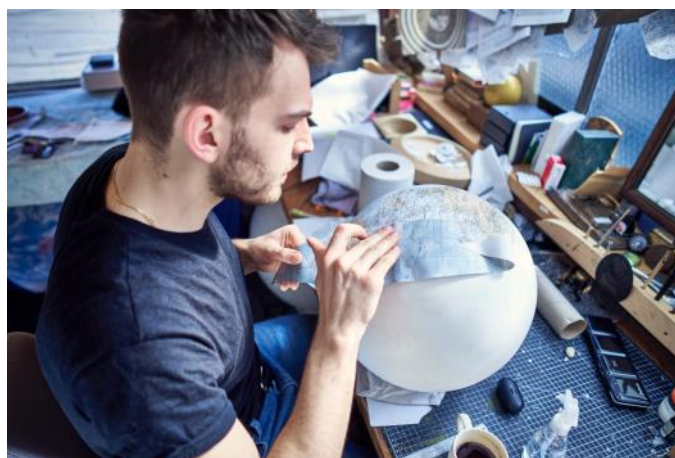
Figure 1. Applying a gore. Image courtesy of Bellerby Globemakers, Euan Myles Photographer.
