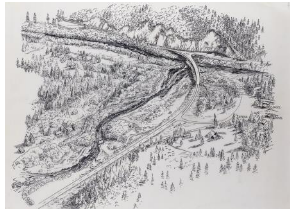
Figure 2. Example of drawings made for Caltrans showing various road alternatives. Sometimes scale models were created to show the proposed road changes and may have been used for design concept approvals and legal negotiations. Photo courtesy of Paul Woodford.
