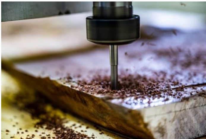
Figure 2. The ShopBot PRSAlpha CNC machine cuts the surface of the sea floor around the Hawaiian Islands into a slab of Claro Walnut. (Photo by Grant Kaye)
