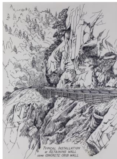
Figure 3. One of several retaining wall illustrations prepared for Caltrans. This type is a concrete crib wall. Image courtesy of Paul Woodford.
