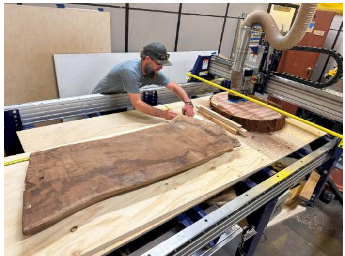
Figure 4. Mike Crabb readies a slab of walnut to be carved into a map of the Hawaiian Islands on the ShopBot. (Photo by Grant Kaye)
